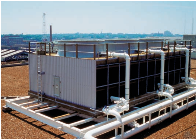
Marley Sigma Cooling Tower —These highly-efficient, low-maintenance towers offer a wide choice of solutions for medium to heavy industrial plants and large HVAC applications. Available in wood (Douglas fir or redwood), steel (stainless or galvanized), or pultruded structural fiberglass for unsurpassed quality and reliability. Tower cells range from 90 to 2,295 m 3 /hr capacities.
